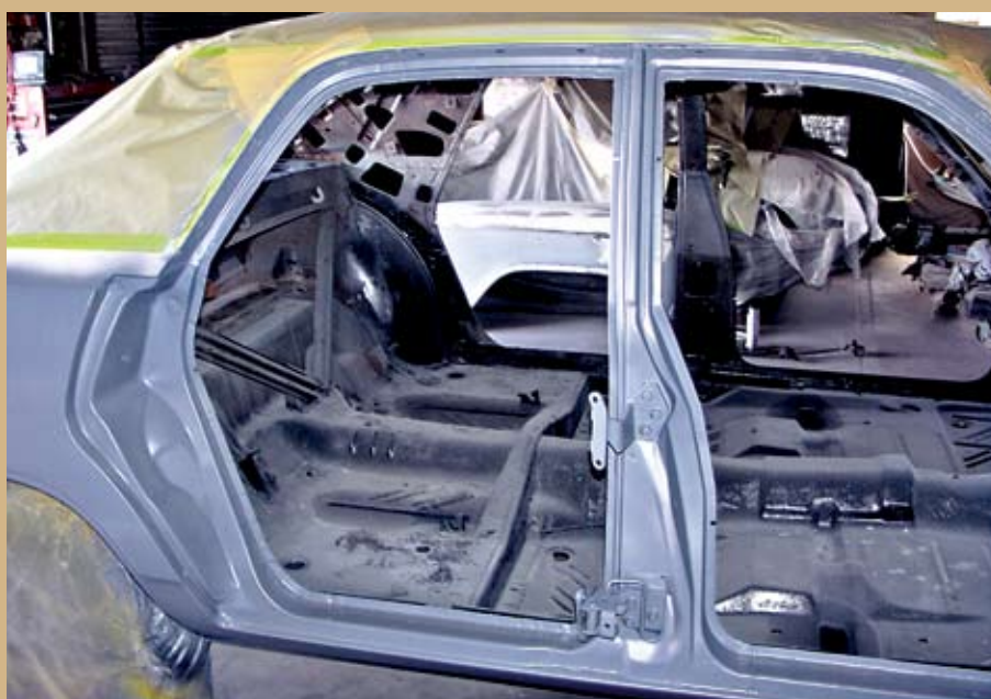
Here the body is primed; roof is taped off to avoid overspray; the white paint has been applied and the painter has prepared the door jambs and quarter panels for the black paint to be applied
