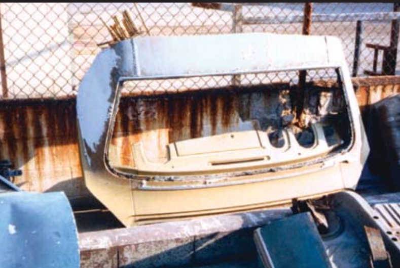
Donor parts car was chosen for rust-free roof to replace rotted one; hours were spent carefully grafting in used section to seamlessly blend with body
