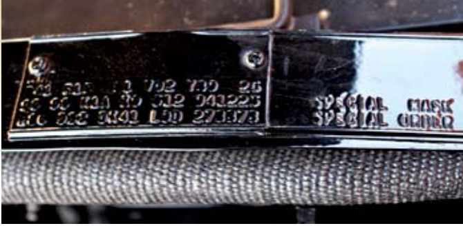
Right fender tag shows “special order” and “special mask” for paint
