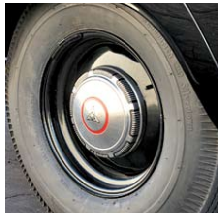
Dog dish hubcap covers black steel wheel and tire
