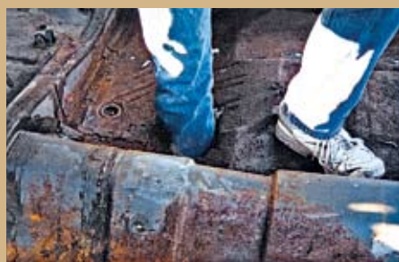
Rusty floors not seen by many Californians; Polara footwell sheetmetal can be scarce
