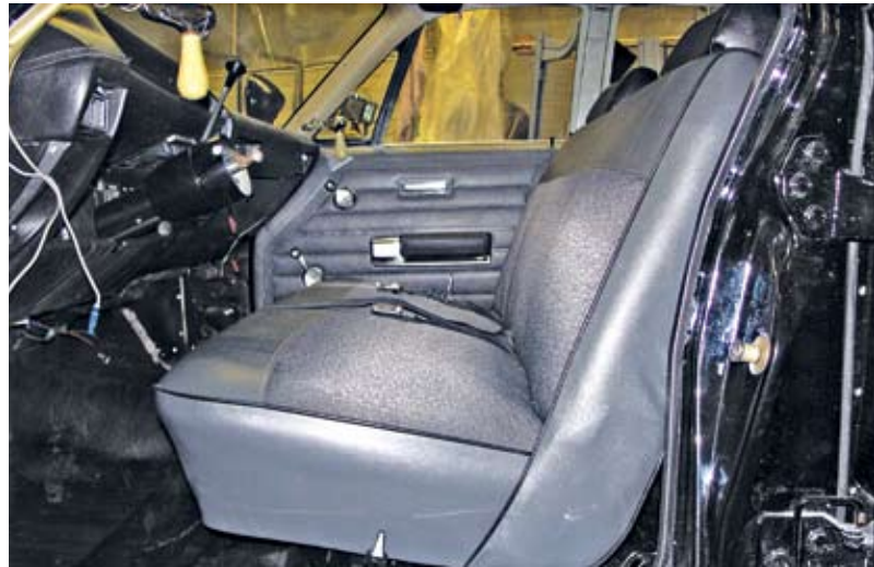
NOS seat and floor materials were found; door panels were refurbished and period-correct lighting installed; ivory spotlight handle is also CHP-spec
