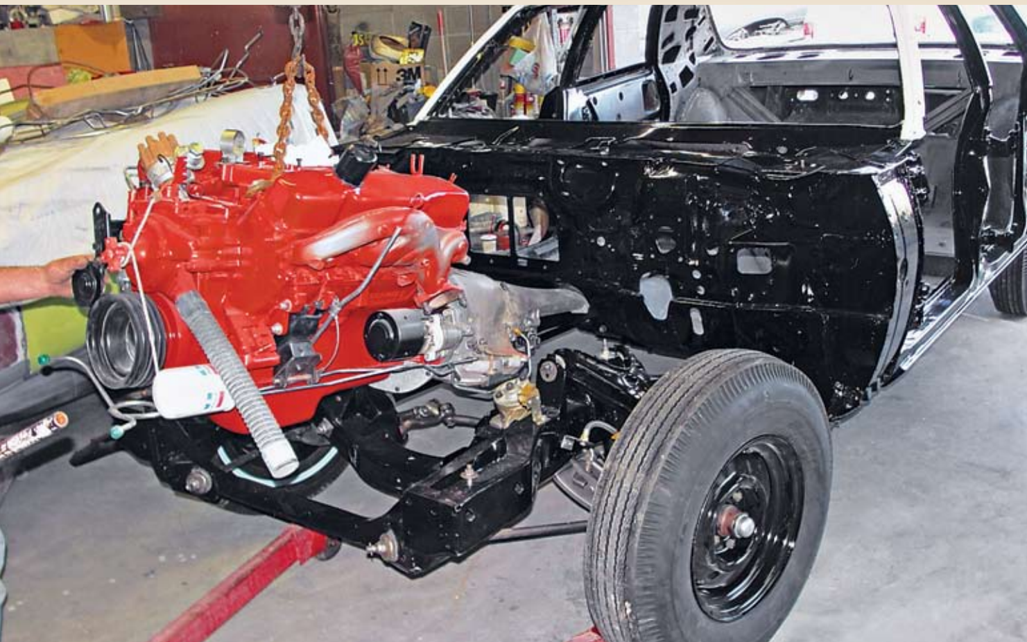
Milestone: the rebuilt and detailed engine being lowered into the restored frame; the remaining sheetmetal was then bolted to the car and aligned to fit
