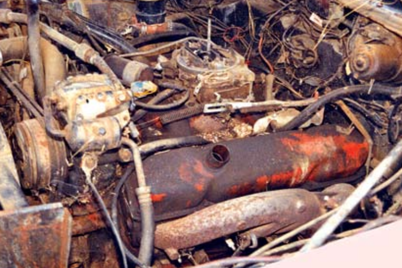
The police-spec 440 presumably had quite a hard life, judging by the level of neglect apparent here; the correct Carter AVS carburetor was missing
