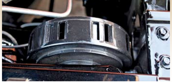
Siren, better known as the “growler,” is mounted to the radiator support
